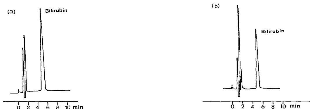
Fig. 2. HPLC separation of bilirubin IX \alpha ; (a) Standard; (b) in serum of a patient with unconjugated hyperbilirubinaemia: column, Hypersil-ODS; mobile phase, acetonitrile-DMSO-water (40:40:20); flow-rate, 1 ml/min; detection, 450 nm.
